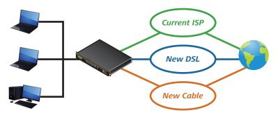
The Peplink Balance Multi-WAN router lets you transparently connect up to 13 Internet links to your existing network. All traffic is automatically balanced and optimized by intelligent algorithms.
