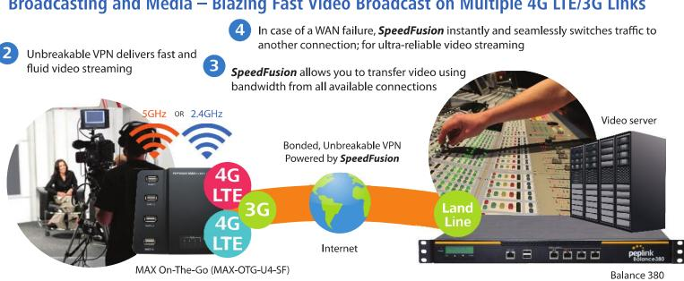
SpeedFusion creates an unbreakable, high-bandwidth connection using multiple USB 4G LTE/3G modems from different carriers
